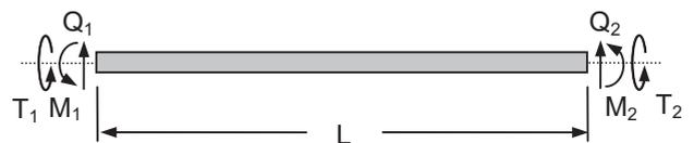
Fig. 2. Boundary forces for a composite beam.
