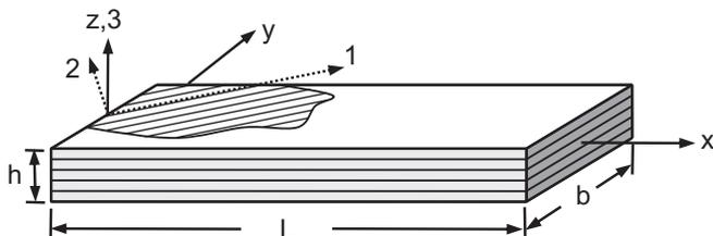
Fig. 1. The geometry and coordinates for a composite beam.
