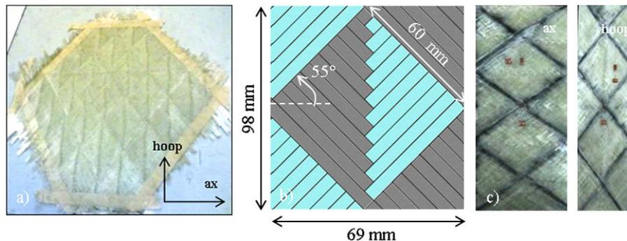
**Fig. 1.** FWC flat specimen (a) pre-form with filament winding pattern, (b) unit cell dimensions, (c) specimens in hoop and axial direction of the pattern.
