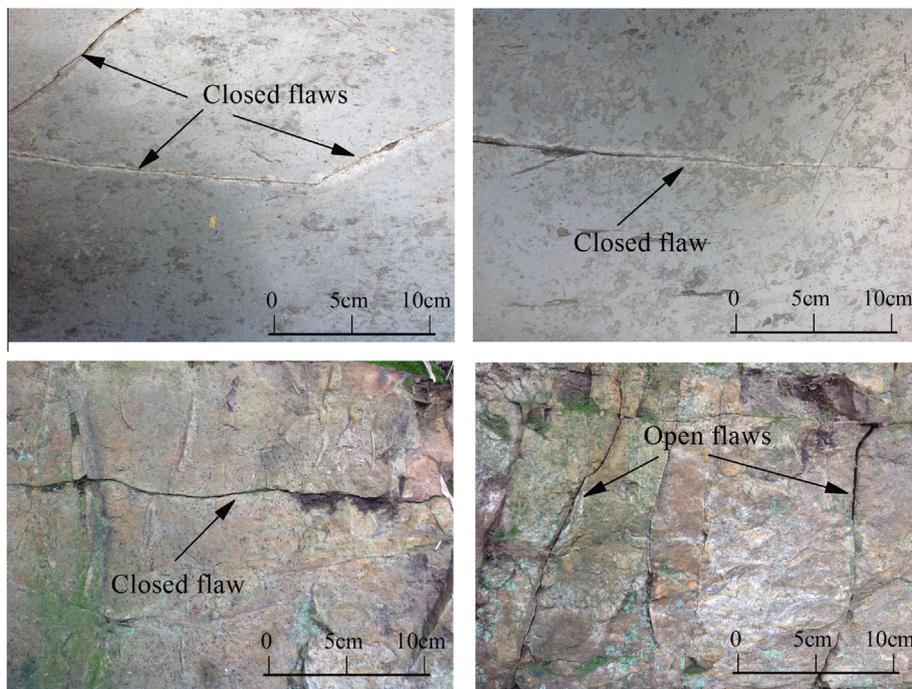
Fig. 2. Open flaws and closed flaws in rock masses.
