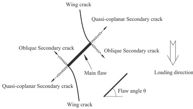
Fig. 1. Crack types observed in pre-cracked specimens of rock materials under compression [4].
