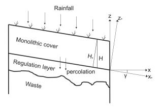
Fig. 1. Schematic diagram of a monolithic cover.
