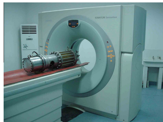
Fig. 2. Triaxial test system with CT scan.
