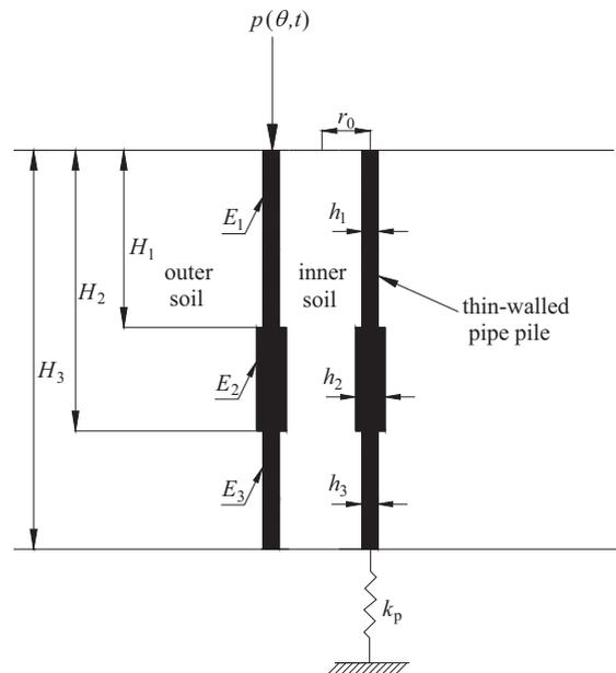
Fig. 2. Conceptual model of the pipe pile-soil system.
