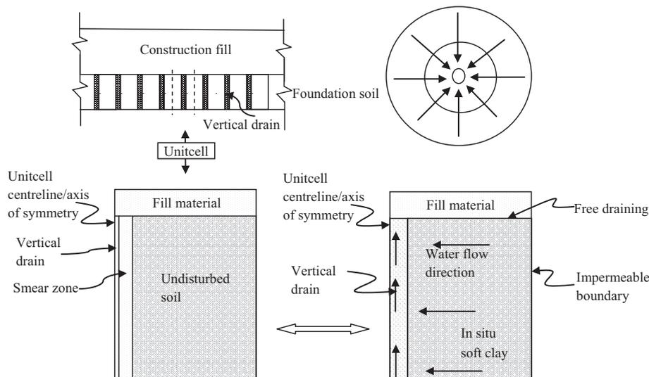
Fig. 1. Unitcell idealization and flow direction of water in a unitcell (not drawn to scale).
