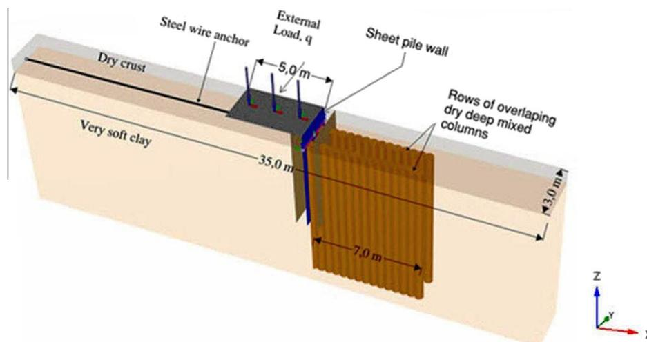
Fig. 1. Model geometry.
