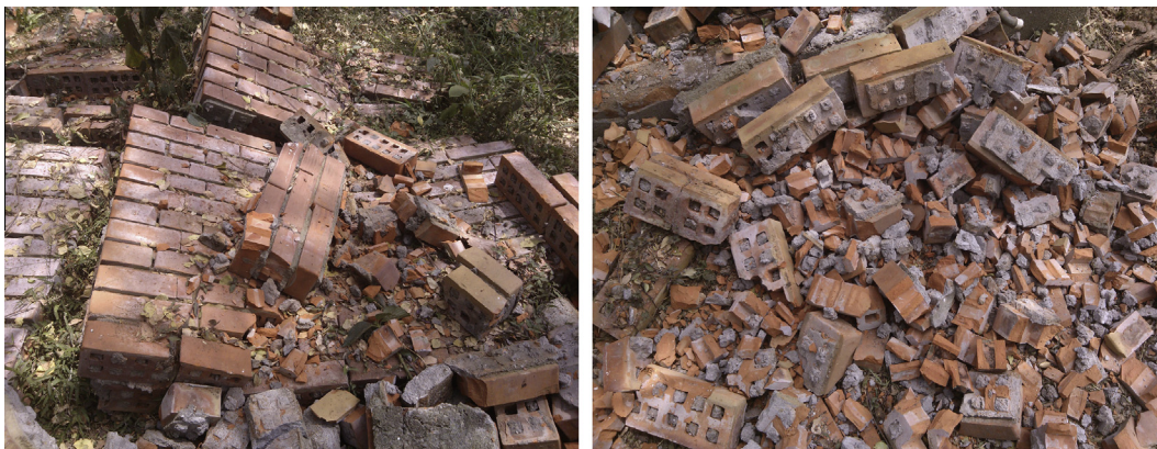
Fig. 2. Residue of masonry (RM).
