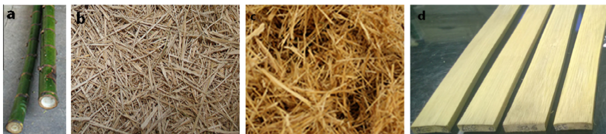
Fig. 1. (a) Water-treated bamboo culms; (b) mechanically attained air-dried fiber bundles; (c) washed BFs reinforcement just before use; (d) BSs reinforcement.
