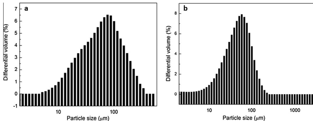
**Fig. 1.** Particle size distribution of (a)  $\text{D-MgO}$  and (b) KDP.
