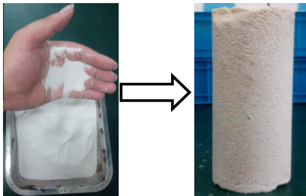
Fig. 1. Loose sand particles to bio-sandstone cemented by bio-phosphate and carbonate composite cement.
