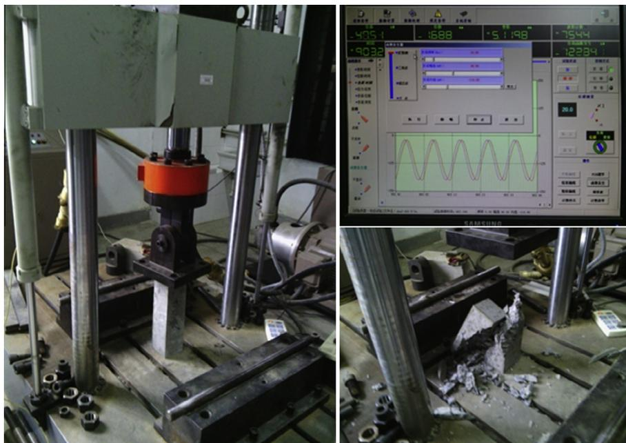
**Fig. 1.** Equipment of compressive fatigue test.
