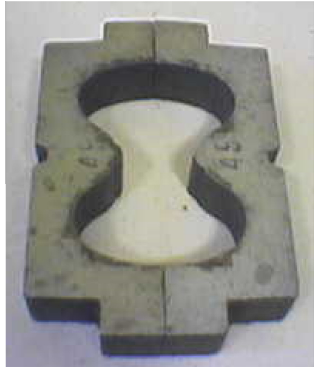
Fig. 2.1.2. Pull-out test specimen Mould.
