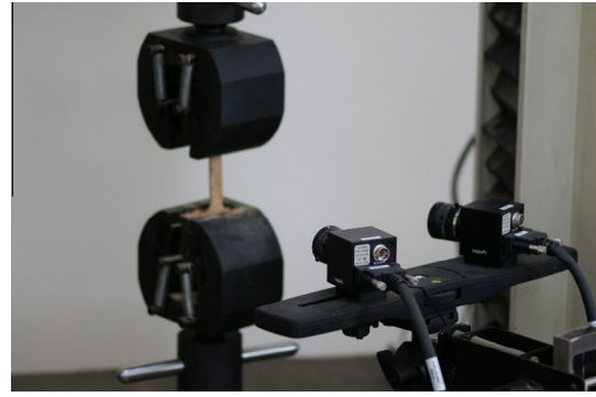
Fig. 2. Digital image correlation testing set up showing two cameras, stereo plate, and tension specimens.
