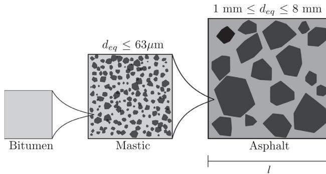
Fig. 1. Different scales for asphalt concrete.
