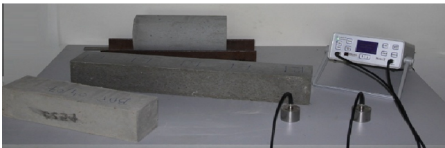
Fig. 1. Ultrasonic test equipment.
