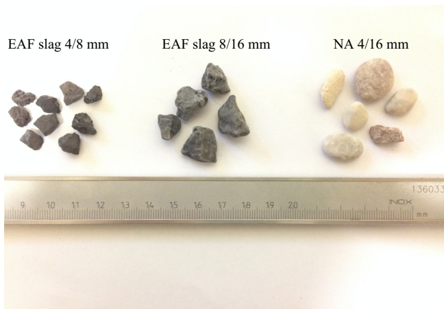
Fig. 1. Appearance of Electric Arc Furnace (EAF) slag compared with Natural Aggregates (NA).
