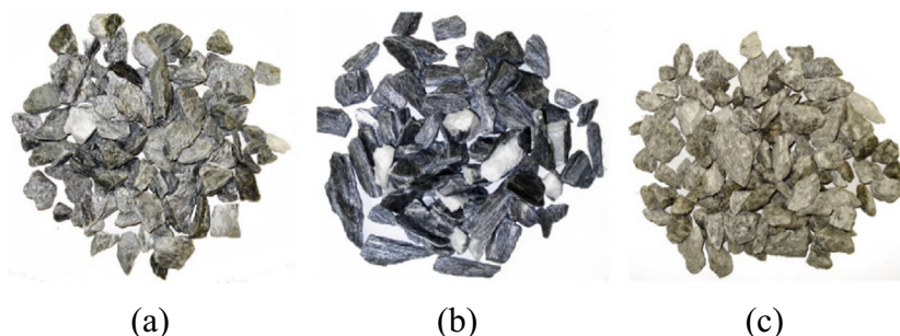
Fig. 1. Investigated excavation materials: (a) quartz phyllite, (b) schist and (c) central gneiss; particle size 8/16 mm.
