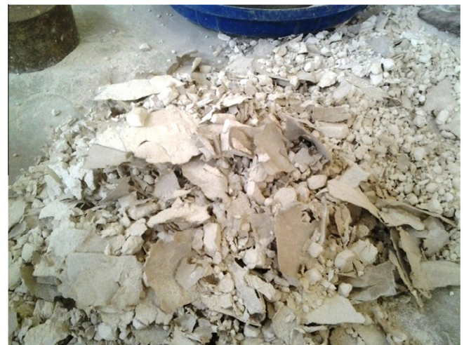
Fig. 1. Waste pieces of gypsum wallboard.
