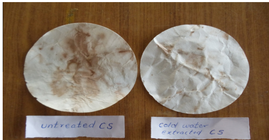
Fig. 1. Iron staining materials in CS.
