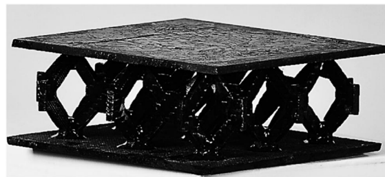
lattice core sandwich panel
