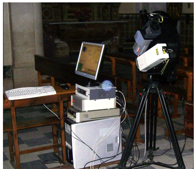
Fig. 1. ENEA LIF scanning system operating in the chapel of San Agustín in Marchena. Computer control on the left, the rotating wheel for vertical scanning, on which the laser and the detector are mounted, on the right, above the tripod.
