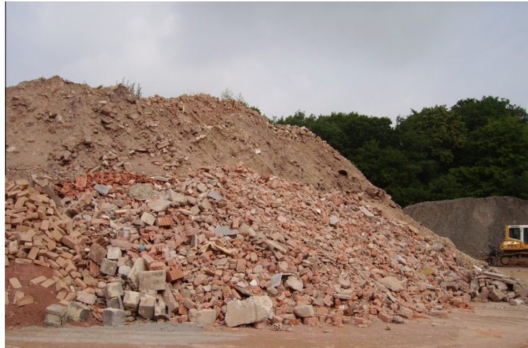
Fig. 1. Example for the input pile of masonry rubble at a recycling plant.
