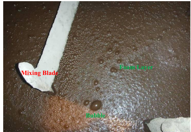
Fig. 1. Small bubbles in fresh CAM with poor bubble stability combine with each other to form into big bubbles and then emerge from the internal to the surface of CAM in mixing device resulting in the formation of bubble foam layer on the surface.
