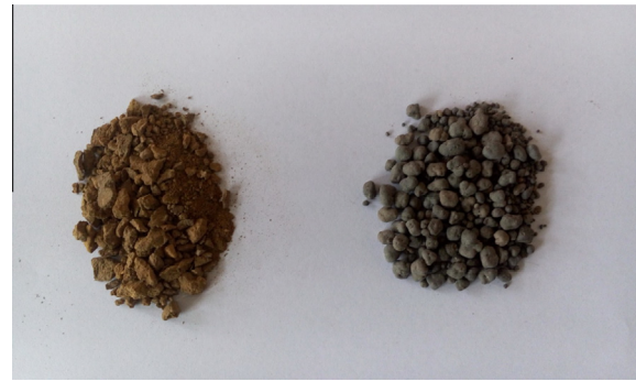
Fig. 1. NWPA and expanded clay. Note: Left one is NWPA; right is expanded clay.
