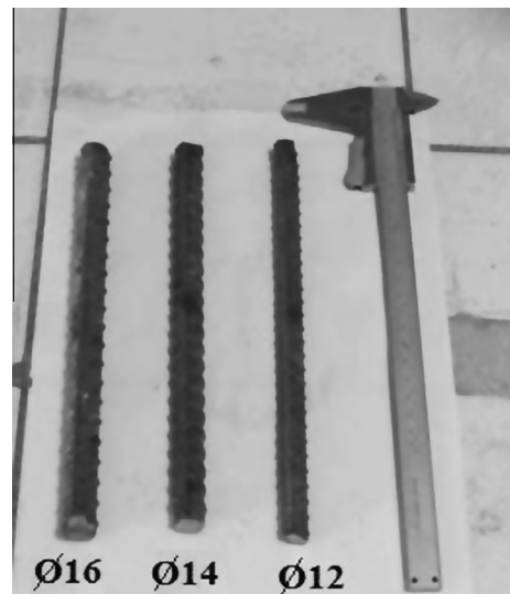
Fig. 2. A view of reinforcement steel rebars.
