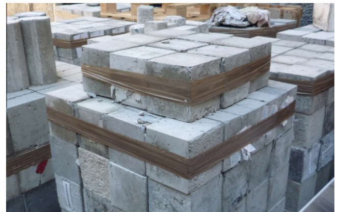
Fig. 1. Concrete wastes before crushing process.
