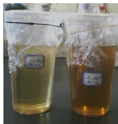
Fig. 1. EMP mixtures with different contents of PU (left: 10%, right: 50%).
