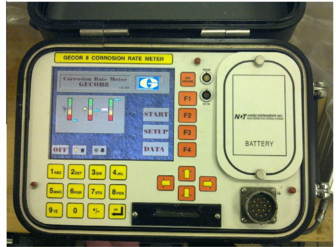
Fig. 3. GEOR 8 for corrosion measurements ( I_{corr} and E_{corr} ).
