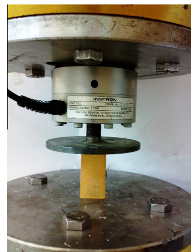
Fig. 1. A composite sample with 60 mm height under loading by an Instron 8802.
