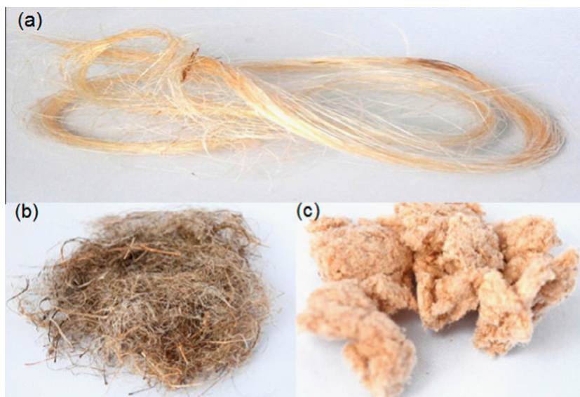
Fig. 1. Images of vegetable fibers in different forms: (a) strands, (b) staple, and (c) pulp.
