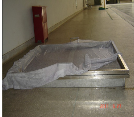
Fig. 1. The strainer for separation carbon fibers from the dispersant solution.
