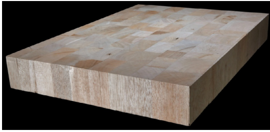
Fig. 1. Balsa panel composed of adhesively-bonded balsa blocks (dimensions 1200 × 1200 × 60 mm).
