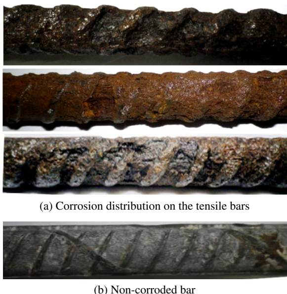
Fig. 1. Comparison of the corroded and non-corroded tensile bars.
