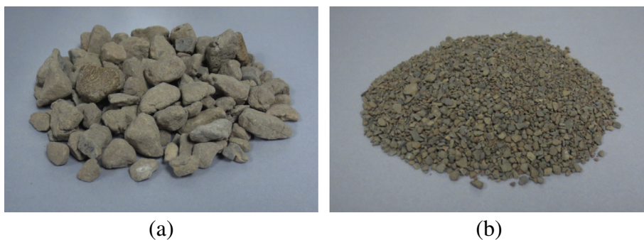
Fig. 1. Artificial lightweight aggregates: (a) coarse aggregates and (b) fine aggregates.
