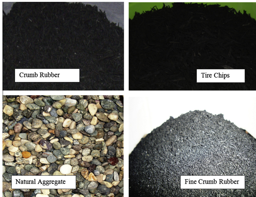
Fig. 2. Rubber materials and natural aggregates used in this research.
