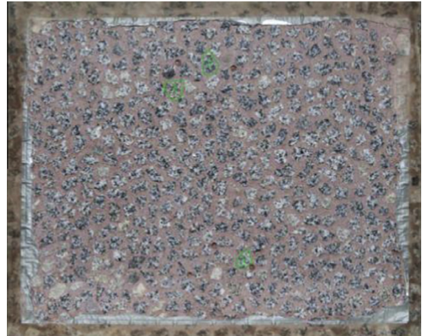
Fig. 2. Test plate of the aggregates [15]. The aggregates are laid over the entire surface of the test plates. Quartz sand is sprinkled into the gaps between the individual grains and concrete is poured over the whole plate. A centimeter-wide rim of the plate is covered with epoxy resin to ensure stability of the edges.
