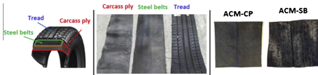
Fig. 1. Description of the parts of the de tire used for the development of the ACM systems.
