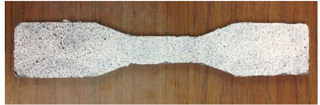
Fig. 2. Random speckle patterns make unique gray scale distributions in each specimen subset.
