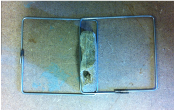
Fig. 1. 2D closed loop fibres interlocking with aggregate.
