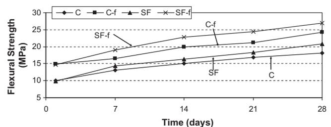
**Fig. 1.** Flexural strength gain of RPC mixtures after standard water curing within time.
