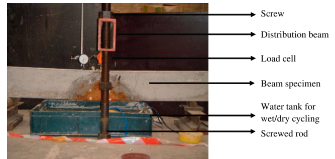
Fig. 2. Test rig for beam loading.
