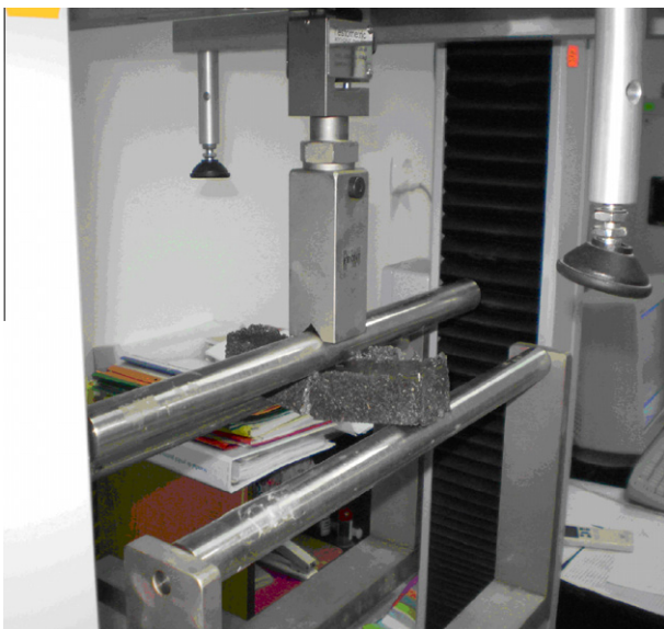
Fig. 1. Polyurethane acryl concrete sample tested in flexure.
