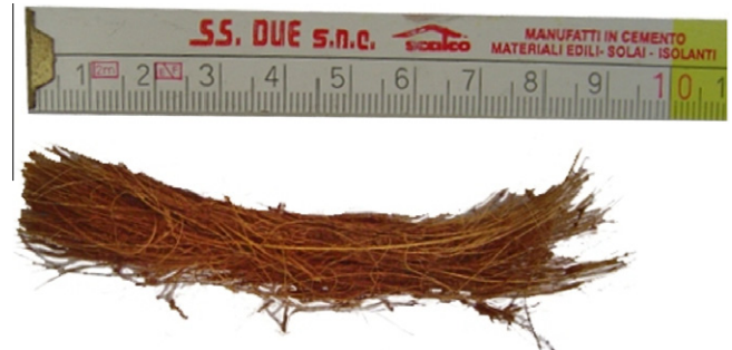
Fig. 2. Coconut fibres used in the experiments as thermal isolating material.
