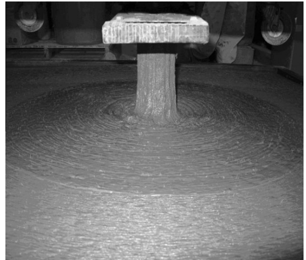
Fig. 2. UHPFRCC placing and flow directions.
