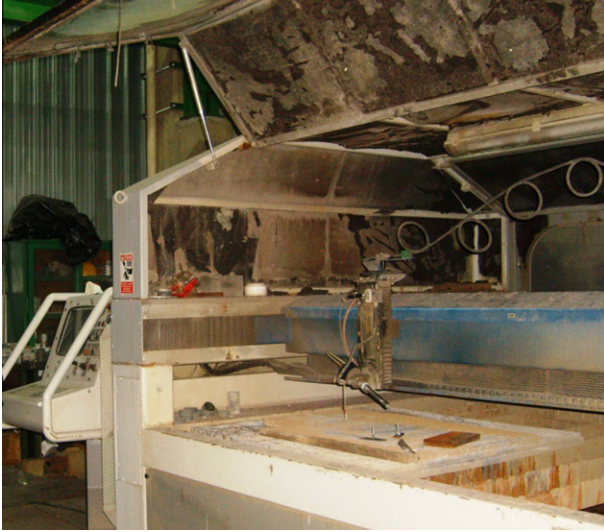
Fig. 1. Water jet machine used in this study (Waterline 1620).
