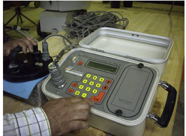
Fig. 2. Half-cell potential measurement assembly.
