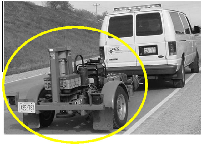
Fig. 1. Falling weight deflectometer (FWD) equipment.
