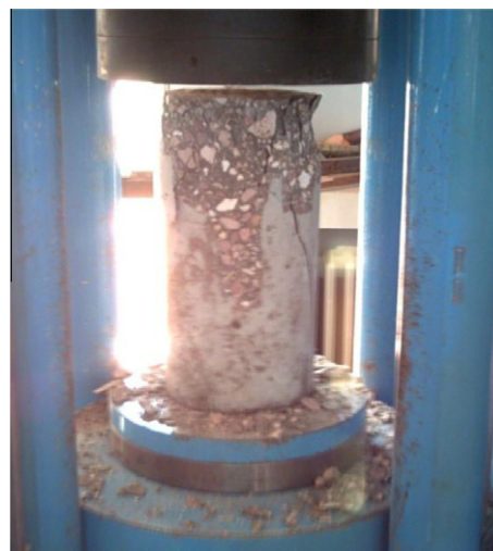
Fig. 1. Concrete specimen in cylinder compression test.
